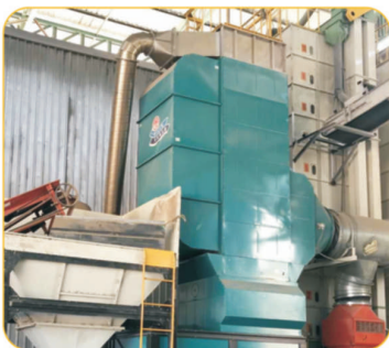
生物质节能稻壳炉 ENERGY-SAVING RICE HULL FURNACE WITH BIOMASS
